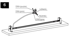
Connect the wires of AC input and dimmer if you have
