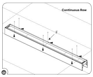
Align all continuous fixtures to ceiling to mark holes and locate J-box (F).
