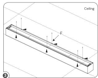
Align fixture to ceiling to mark holes and locate J-box (F).
