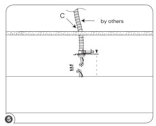
Knockout hole for BX cables (C) and make wire connection to Fixture wires.
