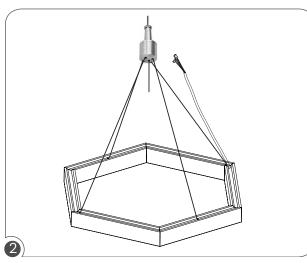
Twist top of the pre-installed gripper to loosen the entrance, insert cables, and lock grippers. Adjust to the desired suspension length.
