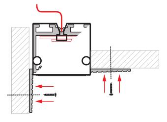
4 Apply a layer of plaster over the flanges and onto the wall to cover the flanges and create an even surface. Do this for both sides attaching to the wall. Once dry, apply paint to finish the surface.
