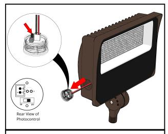
**Step 1:** Unscrew the photocontrol and carefully adjust the switch on the back side to enable or disable the photocontrol. Take extreme care not to pull, pinch, or disconnect the photocontrol wires.
