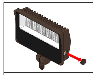
**Step 1:** Remove the conduit plug as shown and set to the desired wattage/CCT.
