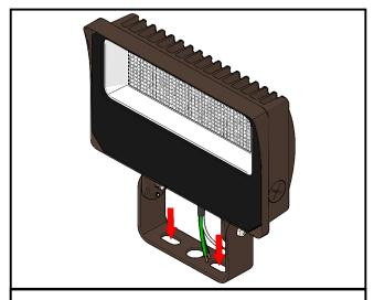
**Step 1:** Mount the fixture to the desired surface using the appropriate hardware (provided by others). Feed the power cable to a junction box or other wiring compartment.
