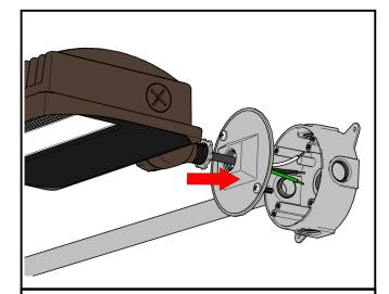
**Step 1:** Feed the power cord into the junction box or conduit. If j-box mounted, insert the threaded portion of the knuckle into the desired knock-out on the junction box. Secure it with the locknut.
