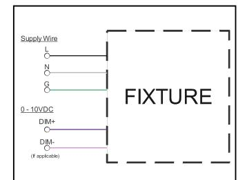
**Step 2:** Make the wiring connections according to the diagram on Page 6. If dimming is not required, make sure the dimming leads are capped.
