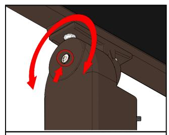
**Step 3:** To aim the fixture, use a hex key to loosen the machine screw on the slipfitter. Move the fixture head to the appropriate position and tighten the screw to lock it in position.
