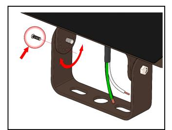
**Step 3:** To aim the fixture, use a screwdriver to loosen the machine screw. Move the fixture head to the appropriate position and tighten the screw in one of the threaded slots to lock it in position.
