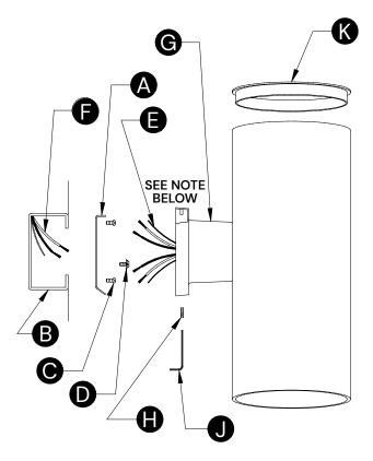
**NOTE**: For up/down light models, wiring connections may be joined for single-switch operation or separated to allow control via two switches.
