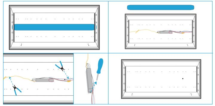
STEP 2: Once the lamps are removed, remove the wiring compartment and disconnect the ballast.
