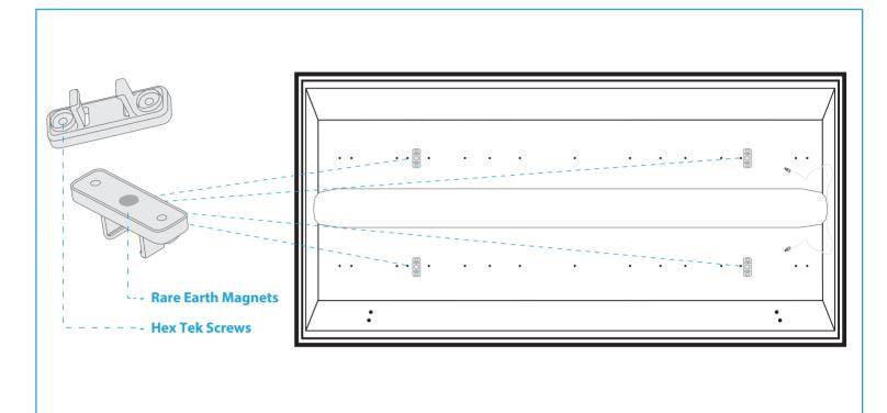
**STEP 5:** Place Infinum Clips into position. Infinum Clips have strong magnets on the back. This allows the clips to be repositionable for perfect easy and pefect palcement. Once the clips are in the desired position, screw them into the fixture using the provided. Hex Tek Screw.
