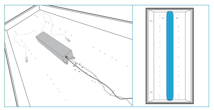
**STEP 4:** Once the ballast is removed replace it with the Quick Connect Driver. The driver is designed to fit in the same location as the previous ballast. Pull the DC lines to the end of the wire compartment. Replace the ballast cover.
