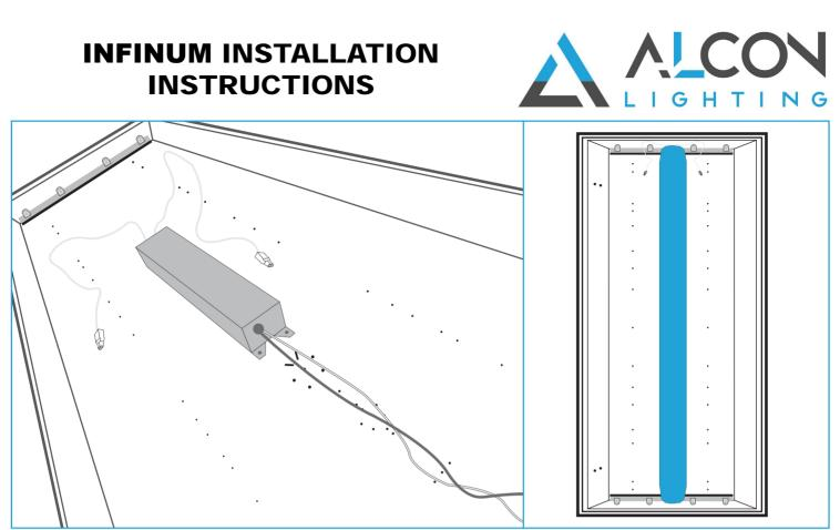
**STEP 3:** Once the ballast is removed replace it with the Quick Connect Driver. The driver is designed to fit in the same location as the previous ballast. Pull the DC lines to the end of the wire compartment. Replace the ballast cover.
