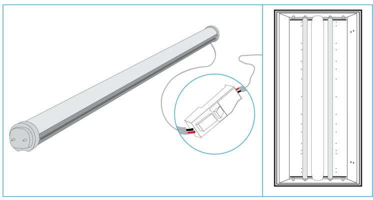
**STEP 4:** Utilize the existing tombstones to hold the Infinum Tubes. Once the tubes are held in place simply connect the quick connects and push the lines back into the wire compartment.
