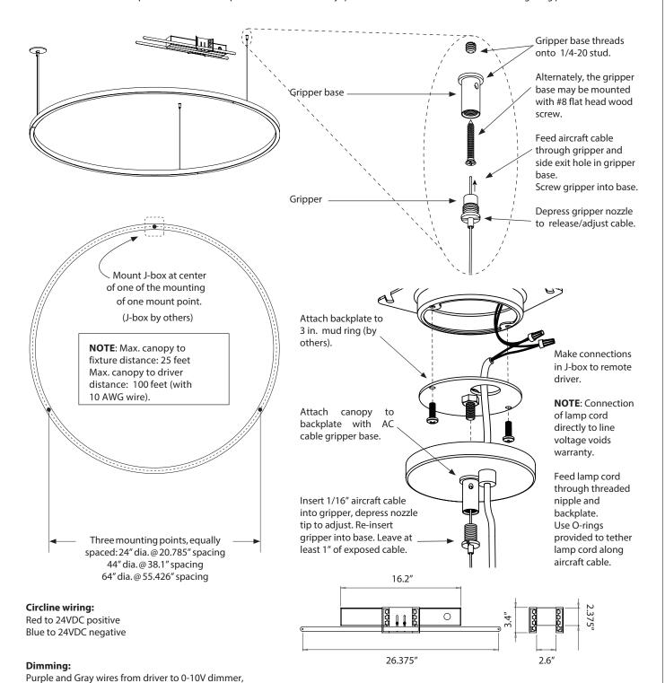
Remote driver includes bar hangers to mount above suspended ceilings. Drivers must remain accessible after installation.
