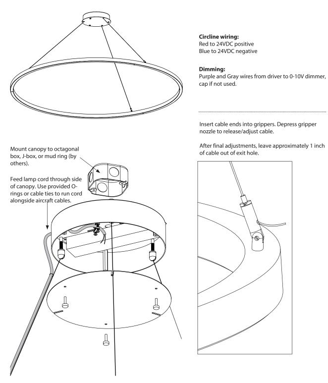
Polarity must be correct for LEDs to operate.
