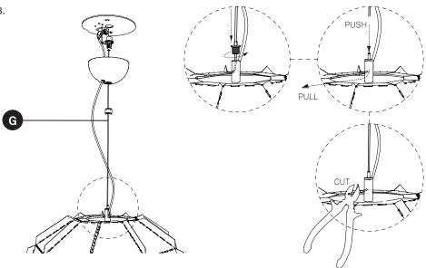
3. Adjust the height of your lamp by raising or lowering the stainless steel adjustment cable (G) and cut off the excess.
