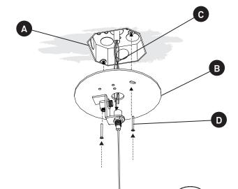
1. The canopy is made up of a back plate with the electrical connections on it and a semi spherical cover.
