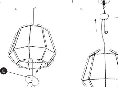
$\textbf{2. Shade Mount.} \, \textbf{A-Pull the Methacrylate plate} \\$ (E) with the light bulb holder on it up through the body of the stitches lamp. It will fit snugly into the top of your lamp. B -Feed the electrical cable up through the frontal sphere (F) of the ceiling canopy.
