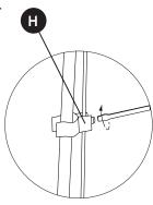
4. Tighten the screw on the electrical cable trap.(F)
